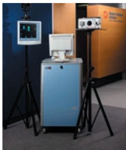
A walk-through thermal scanner originally meant for military use. Image courtesy of Singapore Technologies Electronics Limited Growing Ventures
